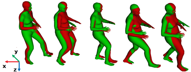
Fig. 7: A qualitative example for predicted pedestrian 3D poses in a walking cycle. The green meshes are predicted by our network and the red meshes are the “ground truth” labels optimized in [21].
