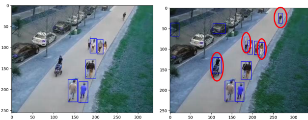
Fig. 1: Visual examples of person detection. Left: CFT with single-frame input. Right: Temporal CFT (proposed).
